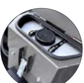
Long range tank with transfer pump
